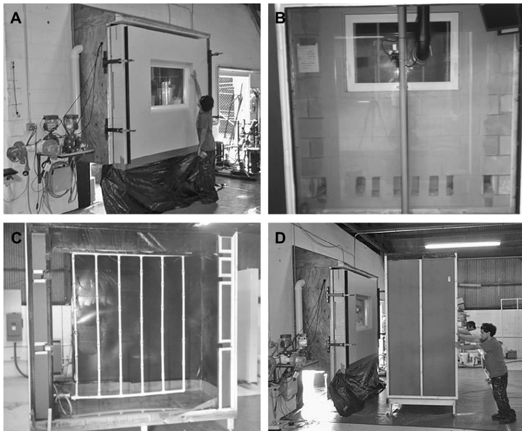
Fig. 6. Negative pressure chamber. A) Test specimen attached to chamber. B) View from interior of Negative Pressure Chamber. C) Wetting chamber containing the calibrated spray rack. D) Wetting chamber is sealed to the front of the test specimen to collect water.
